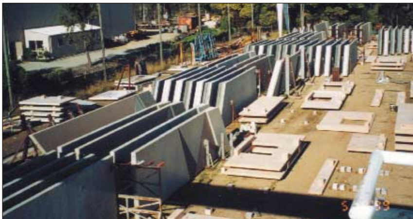
Panels in storage at precaster's yard awaiting delivery (above) and a 12.6 m x 3 m precast panel being transported from factory (left)
