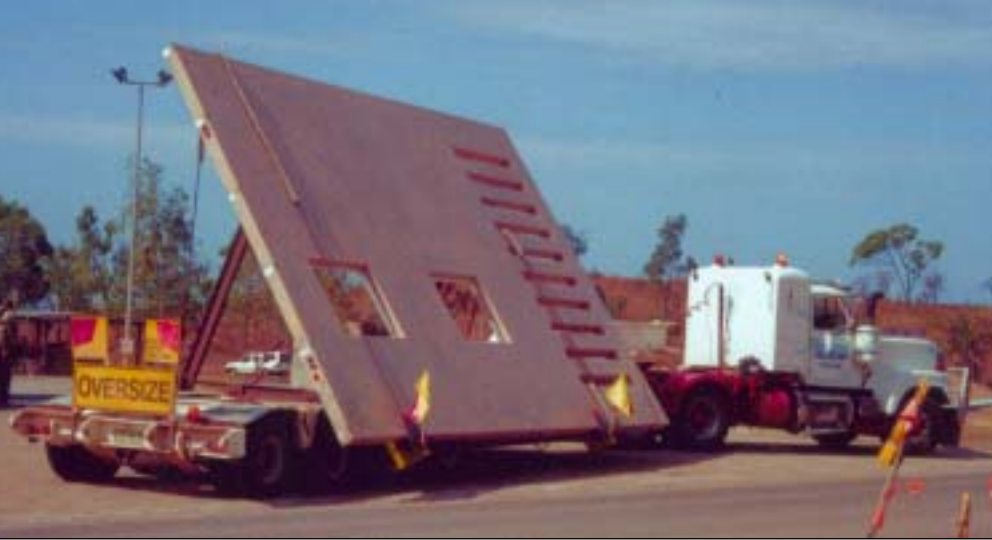
Customised counterweighted transportation rig for overdimensional panels – 11 m long and 5 m wide weighing up to 16 tonnes each
